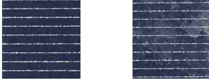
Figure 4.5: Solar panel samples. Left) clean panel; right) dirty panel [87].
